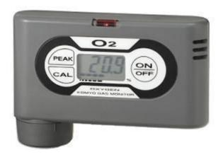
To protect the worker from injury by oxygen deficiency, the oxygen concentration in the air must be monitored. The pocket sized OPA-5000E O<sub>2</sub> Monitor can be carried as a personal monitor or used to measure remotely with the optional extension cord and adapter.
